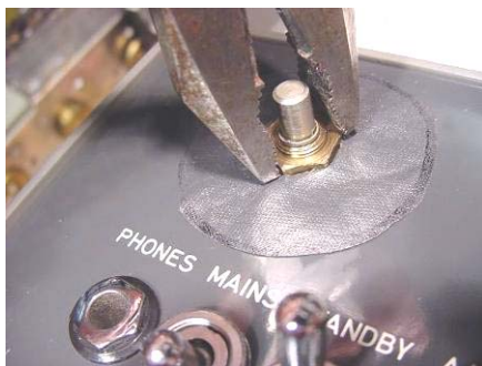
Removing the controls – note the oversized scratch guard
