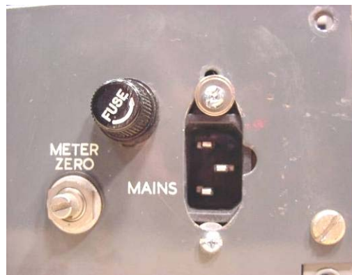
‘Euro-connector’ mains connector now fitted (not much use at present!)
