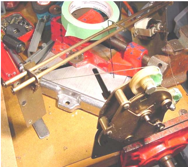
Gearbox in my bench vice for cleaning (note dial cord still attached and threaded through idler and jockey pulleys)
