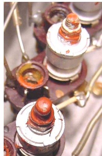
Hardened red sealing wax on the concentric trimmers and coil slugs
