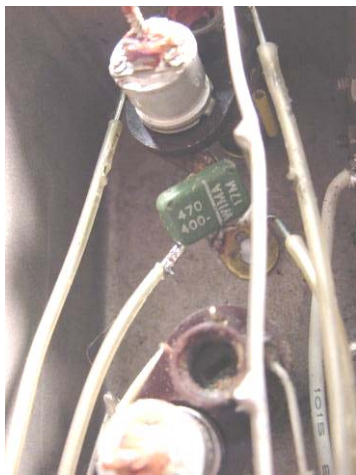
Temporary bridging cap in Band 4 aerial circuit
