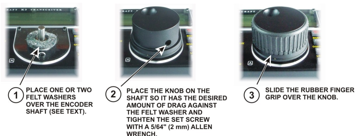
Figure 49. Mounting the VFO A Tuning Knob.
