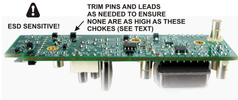
Figure 69. Checking Lead Lengths on KREF3 Board.
