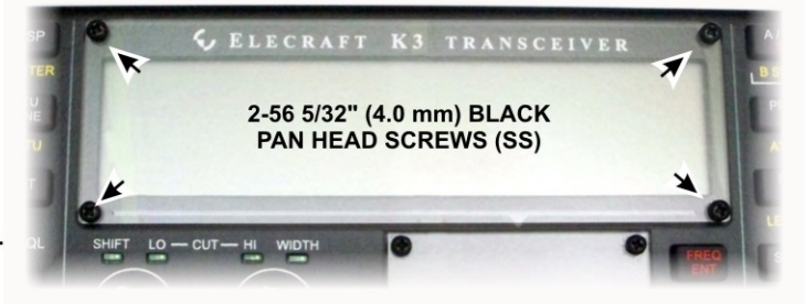
Figure 46. Installing LCD Cover.
