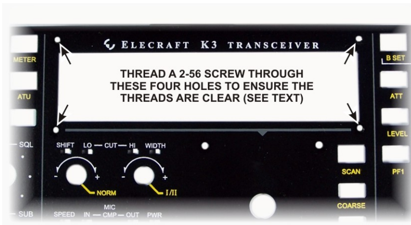
Figure 39. Checking 2-56 Threaded Screw Holes.
