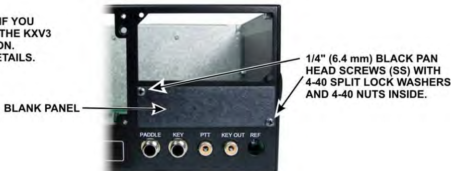
Figure 31. Preparing Rear Panel for KIO3 Installation.
