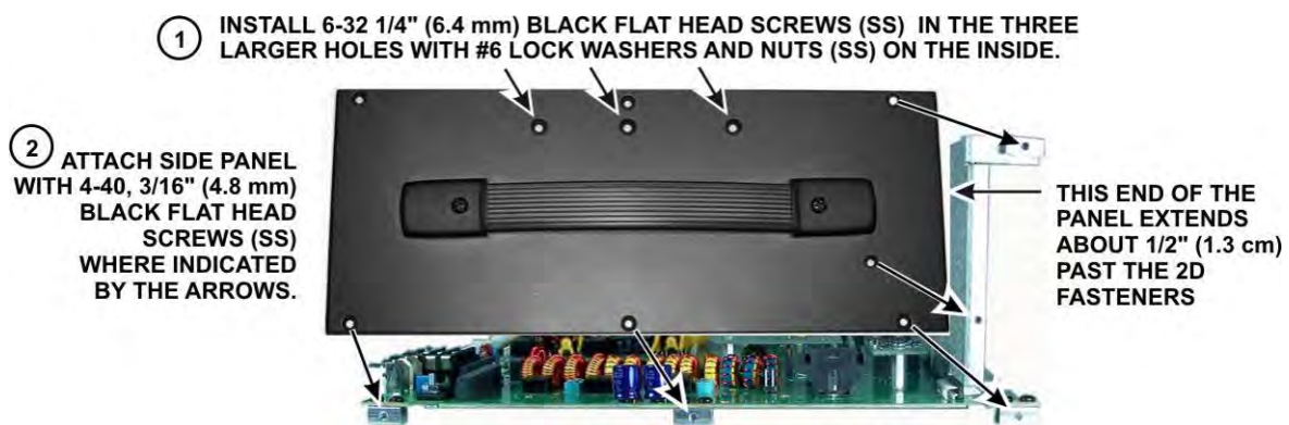
Figure 16. Mounting Left Side Panel.
