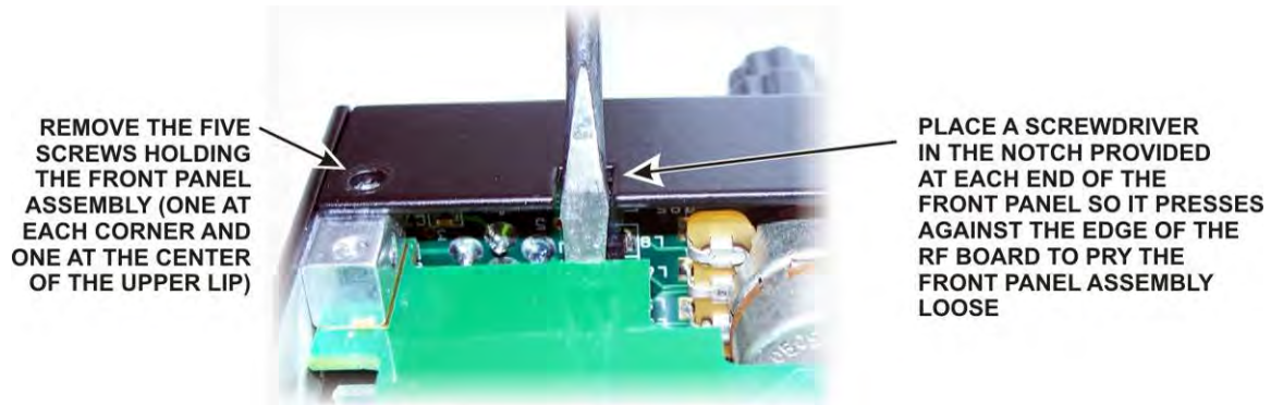
Figure 64. Removing the Front Panel.
