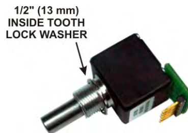
Figure 42. VFO A Encoder Assembly Preparation for Installation.
