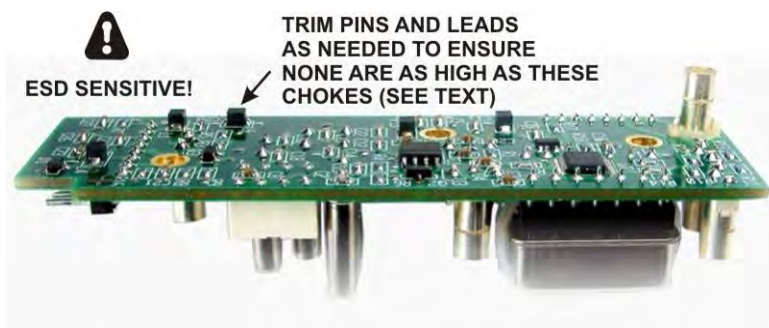
Figure 70. Checking Lead Lengths on KREF3 Board.
