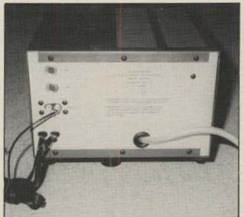
A rear view of the PS-9000. Separate line cords are provided for the power supply/clock circuits and there are two circuit breaker resets (one for each of the two 110 V primary windings on the power transformer).
