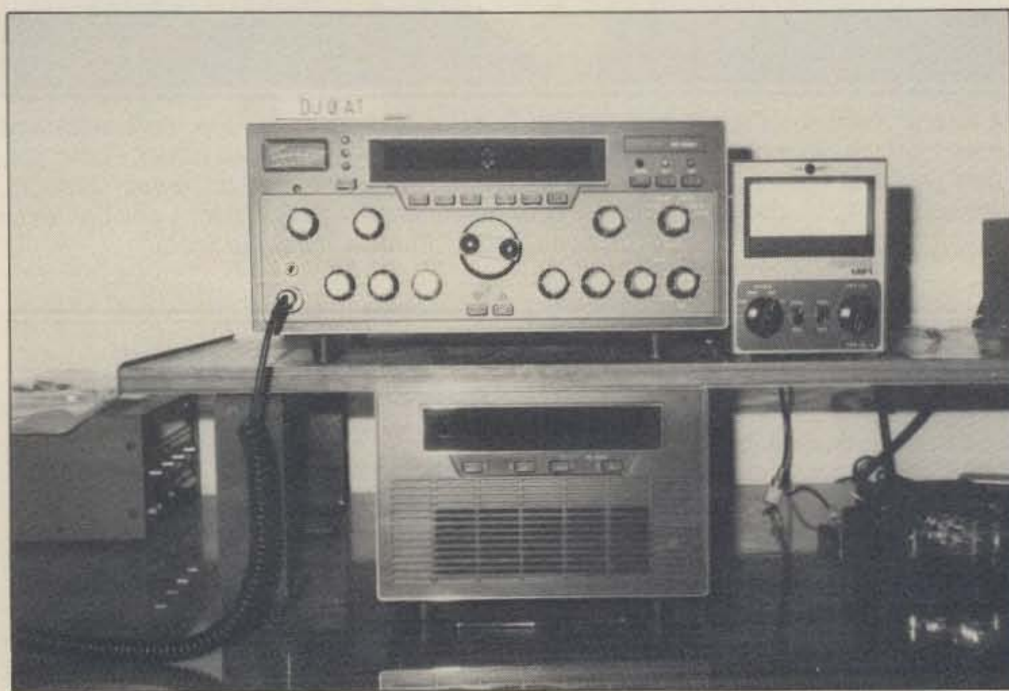
The SS-9000 on the operating table with the PS-9000 power supply below it.
