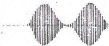
Fig. 6 C 100 % modulation (tone)
