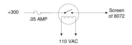
The bias line that is normally controlled by K1 must be shorted (Short A5-259 to A10-5). According to Amperite, there is no problem controlling 300 VDC since heater to ground spec is 800 VDC.
