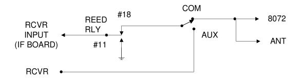
8. To increase frequency response on units that exhibit a narrow response in transmit and receive making tuning difficult:
