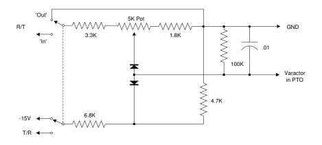
**21.** Addition of Receiver Incremental Tuning utilizing FSK control:
