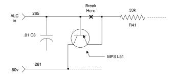
The desired output may now be set with the ALC potentiometer on the A77.
