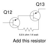
**PROBLEM** 8.8 MHz carrier misadjusted. (R46 on BFO board, A4)
