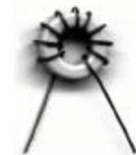
Completed L6 (L7 is the same, but with 1 turn less)
