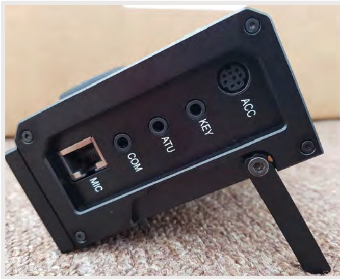
Fig. 1: Side view showing some of the interfaces and one of the feet.
