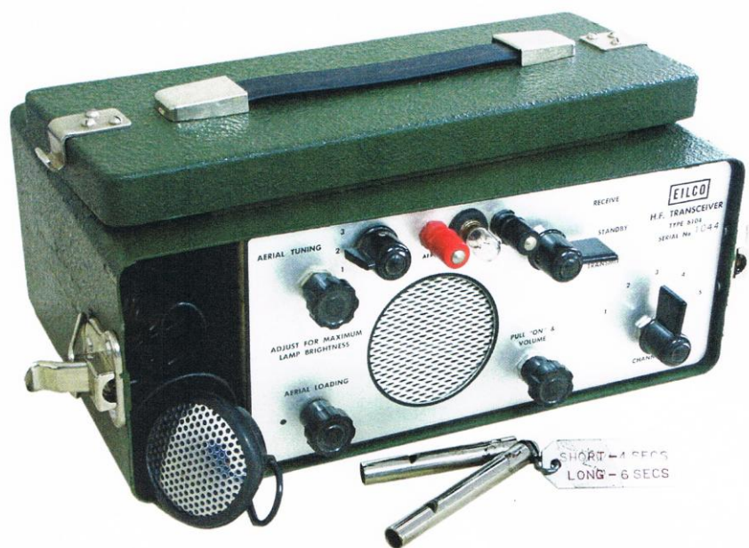
Figure 2 Original type 6104 AM set. Note the two tin whistles to be blown to initiate an emergency call
