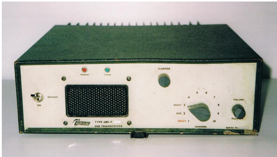
Figure 1 Type 6801 SSB set, 5 channels, 100 watts PEP
