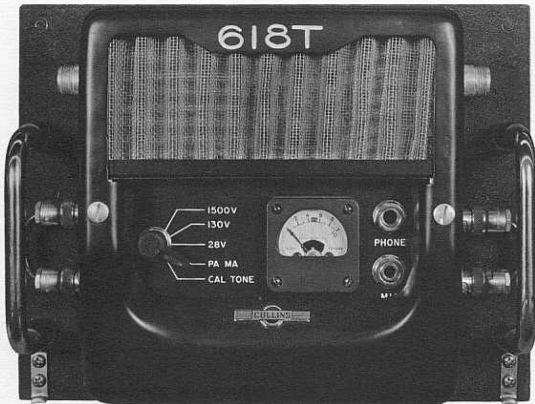
Front Panel Metering
