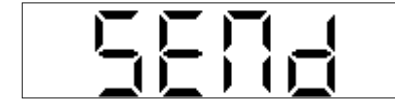
This display shows that the Selcall is being sent - ie. in transmit mode.
