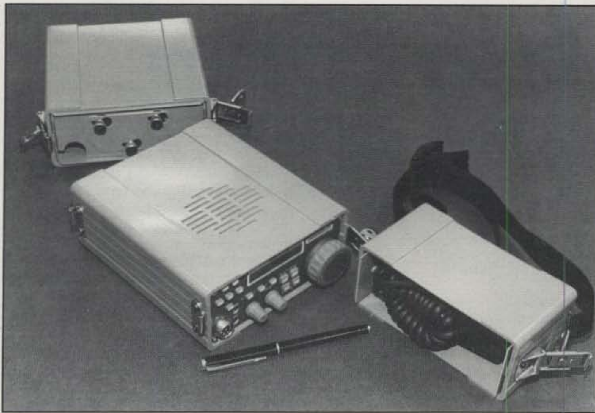
Optional snap-on front and rear covers convert the SG-2020 into a self-contained station that goes with you anywhere and anytime. Batteries install in rear, and microphone and key store in front. (Photo courtesy SGC, Inc.)
