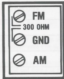
EXTERNAL ANTENNA TERMINALS CABINET BACK VIEW
