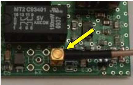
Fig. 31: Detail, MMCX plug
