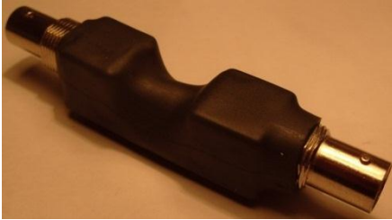
Fig. 163: Covered with Heat-shrink Tubing
