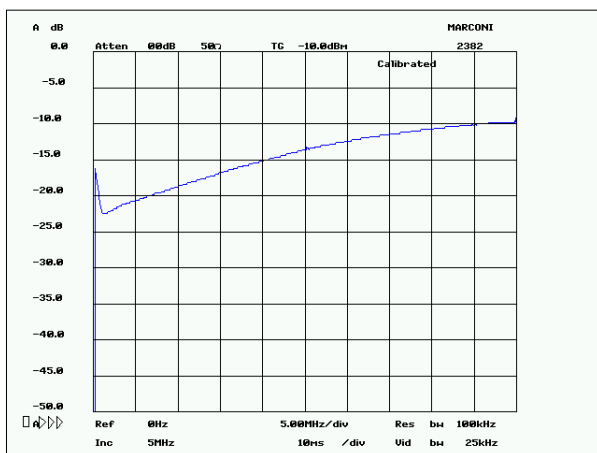
Fig. 173: Return Loss Input without Prefilter (pass-through)
