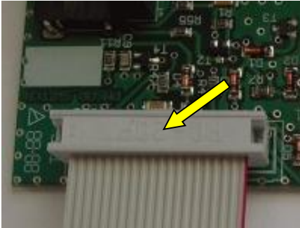
Fig. 30: Ribbon Cable connected
