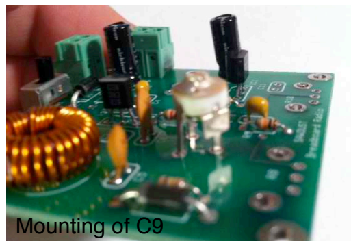
T1 leads tinned and mounted
