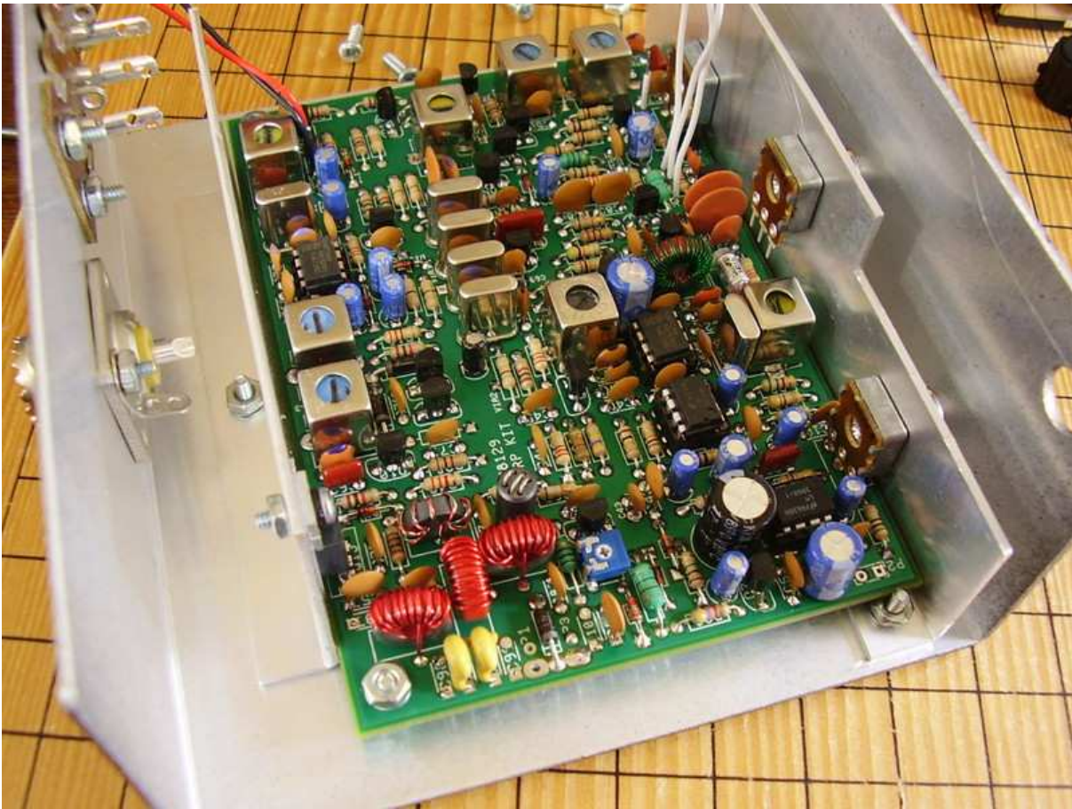
Figure 10.2: Board Installed in Center Shell.
