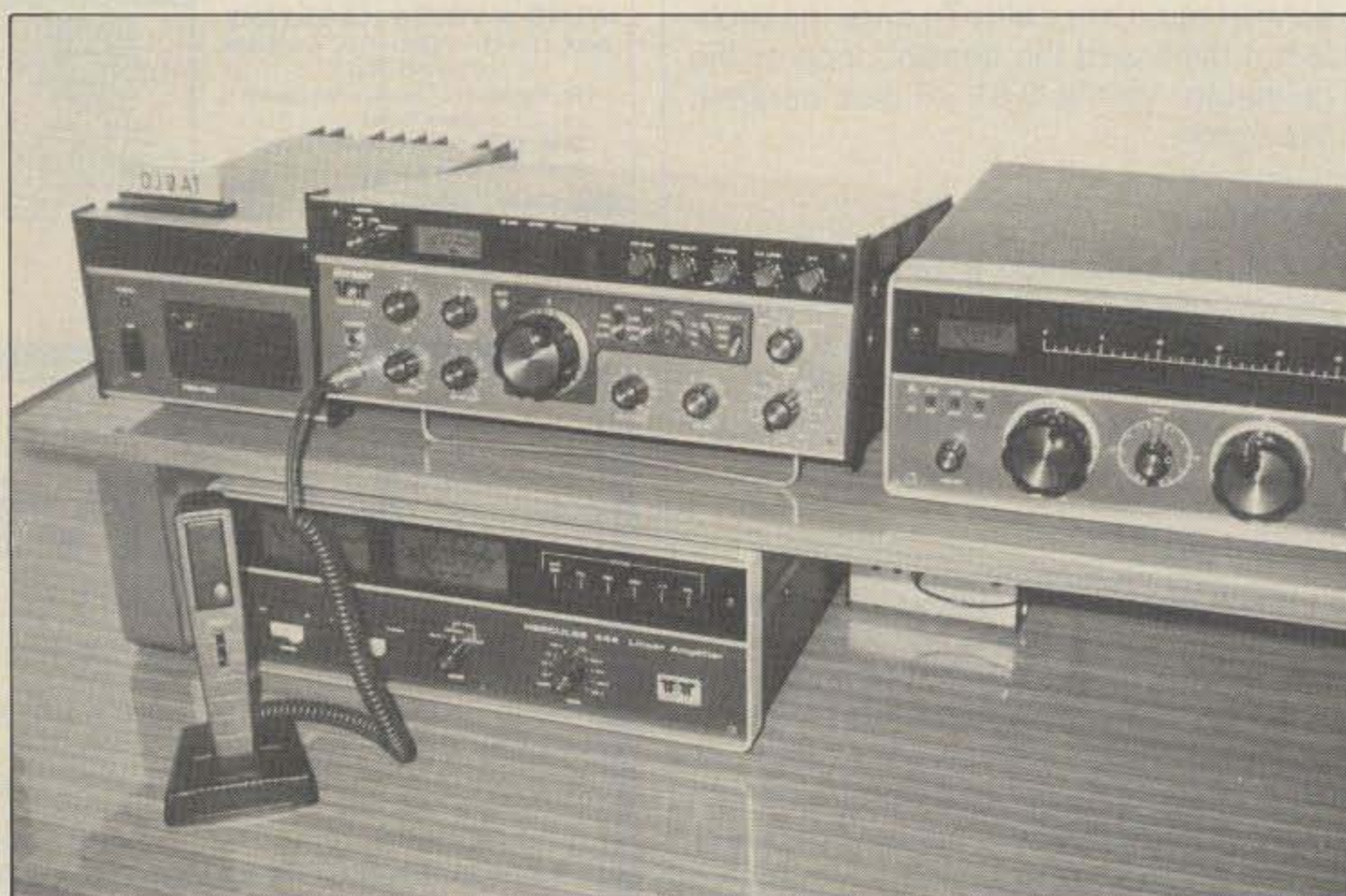
Although the Corsair has new styling, it fits in nicely with other Ten-Tec equipment in this station setup. (The Hercules solid-state linear is below it and the Model 229 tuner is to the right.)
