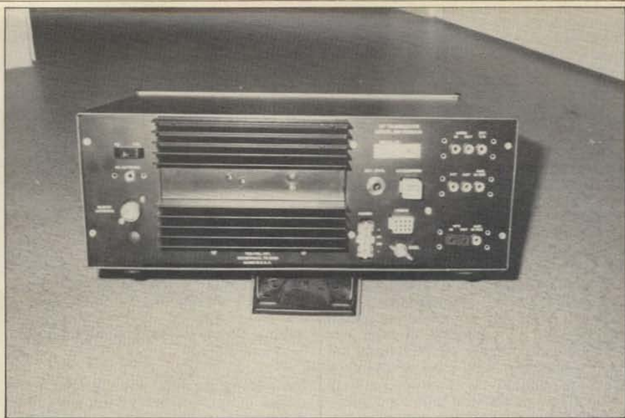
The rear panel is clean and functional. There is no cooling fan, and none is needed for normal c.w./s.s.b. operation. Even after extended operating periods, the heatsink never got more than slightly warm to the touch.
