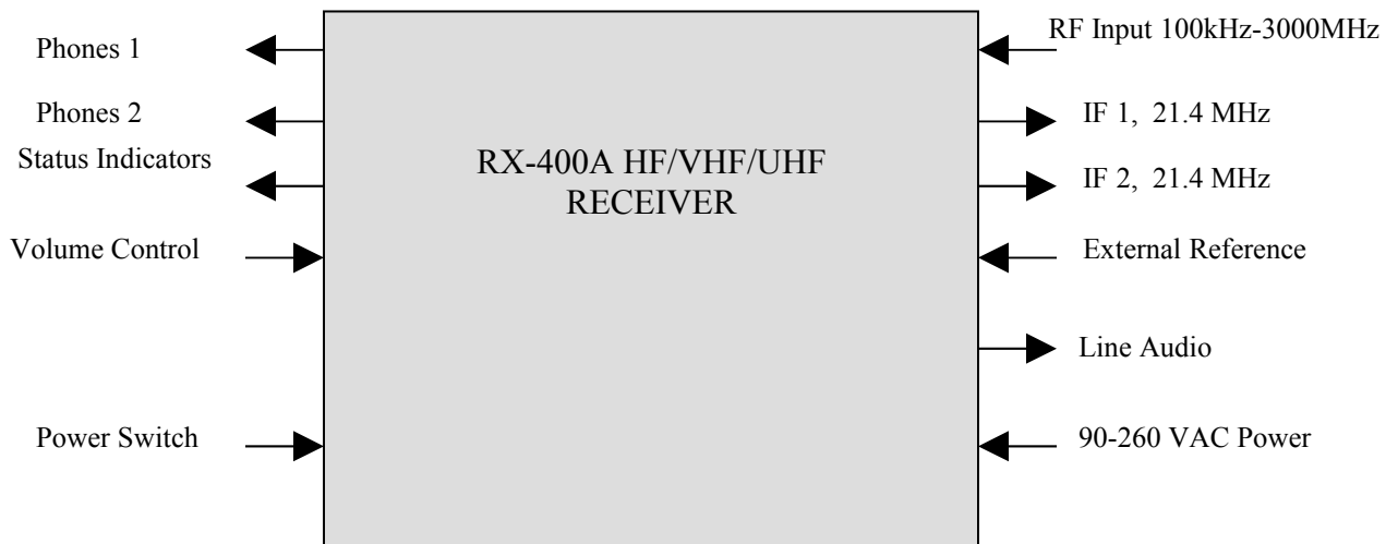
FIGURE 2-6 RX-400A ELECTRICAL INTERFACE
