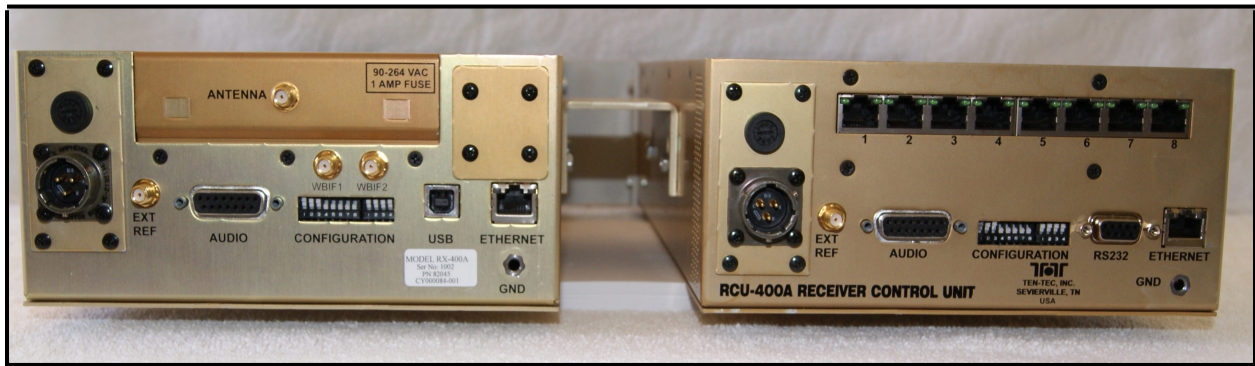
Figure 2-4 RX-400A Receiver Mounted Side-By-Side with RCU-400A Receiver Control Unit Rear View
