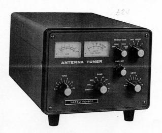
The FC-901 antenna coupler is designed for low and medium power applications in the HF amateur bands from 160 through 10 meters. It is designed to minimize the adverse effects of high SWR on a coaxial line or wire antenna which may result in difficulty in tuning a transmitter designed to work into a resistive 50 ohm load.
