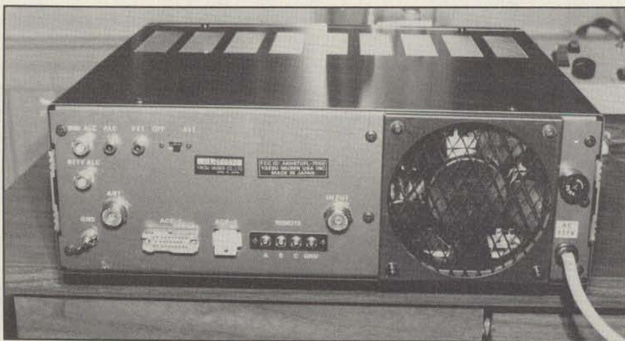
The back panel shows the cooling fan for the power supply plus the various connectors. The terminal strip in the lower middle supplies an operating voltage for up to three external antenna relays which can be switch-selected from the front panel of the FL-7000. Separate ALC-level adjustments are provided for SSB and RTTY (upper left).
