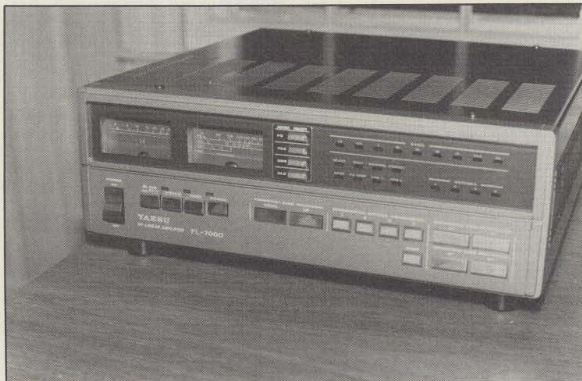
The FL-7000's front panel consists only of various fields of pushbutton controls, LEDs, and two analog meters. If the amplifier is fully set up for automatic operation, only the power on/off switch and the operate/standby switch have to be used.
