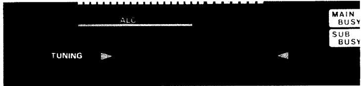
Fig.7-2 CW TUNING METER
