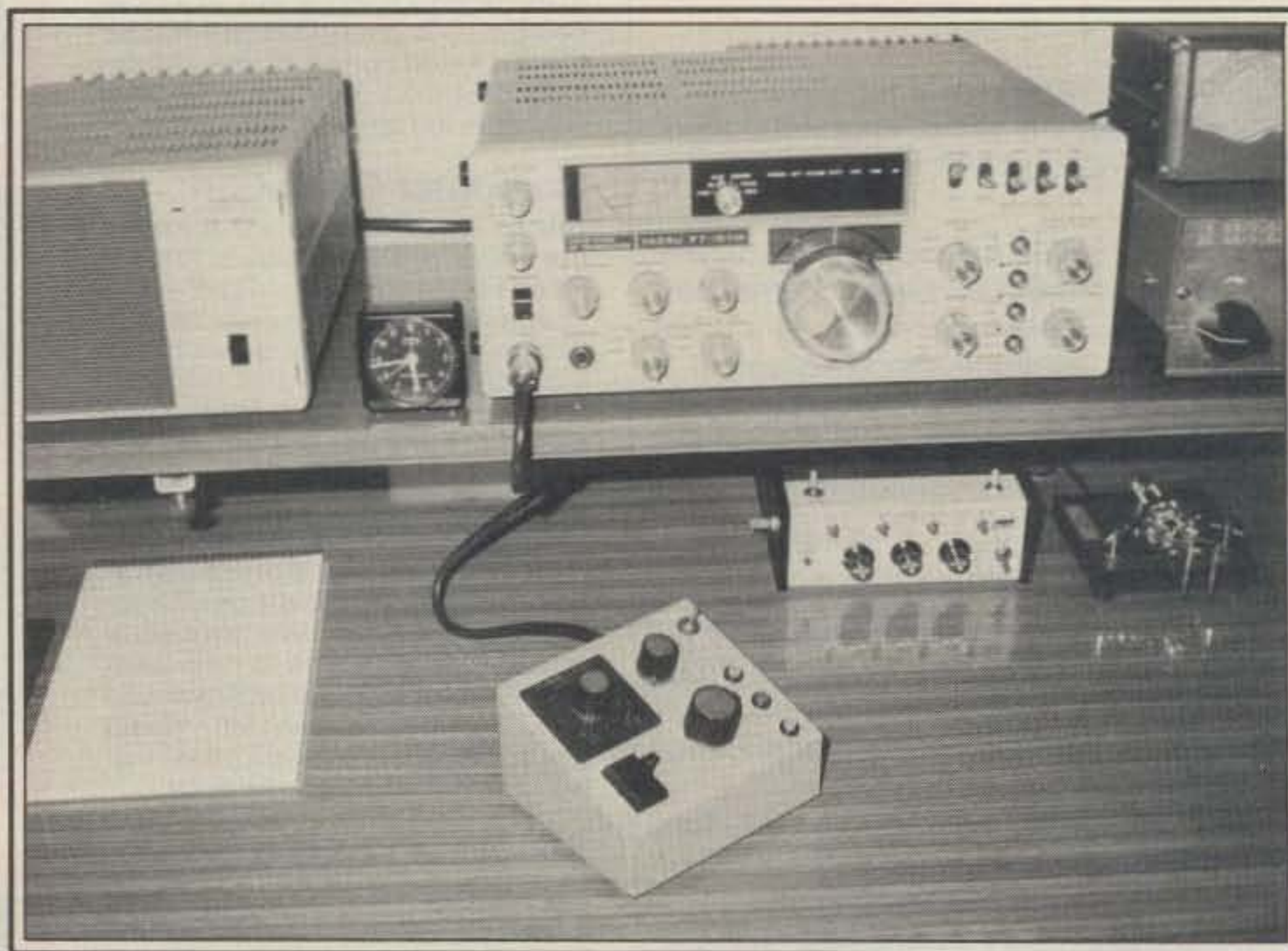
The FT-107M with the FP-107E power supply on the left. The small control box in the foreground basically duplicates the push-buttons found on the optional Yaesu YM-35 mobile scanning microphone so one can effect scanning operation in a home station situation using any microphone.
