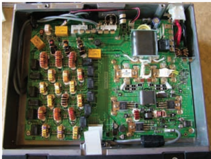
Figs. 2 and 3: Internal views of the FT-40 circuitry, including power amplifier stage.
