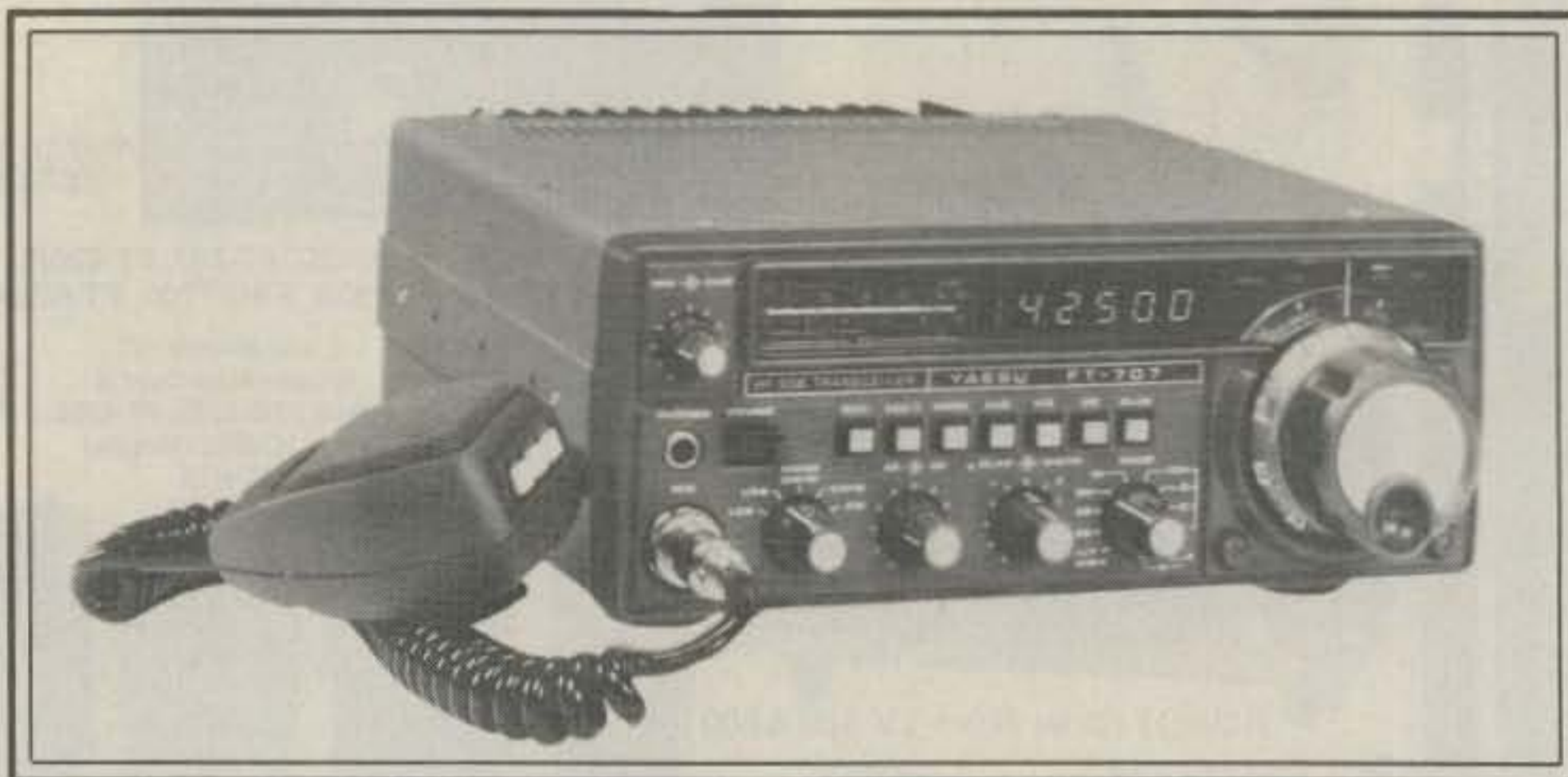
The FT-707 is both handsomely and compactly packaged. It is shown with a scanning-type microphone, but the scanning feature requires the FT-707DM Digital VFO.
