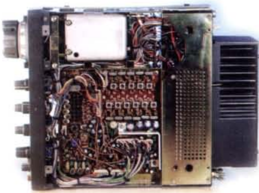
● Fig. 3: Underside view of the main p.c.b. with the massive heat sinking for the p.a. stage on the far right with the shielding (with perforated screening) of the two transistor power amplifier on the near right.
