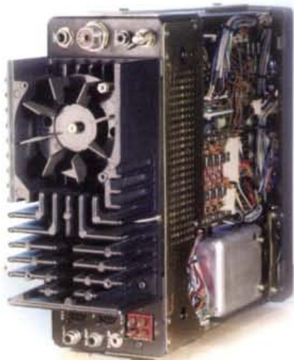
Fig. 4: Rear view of the FT-707 with fan protection and ducting screen removed. Note heavy duty cast aluminium heat-sinking ducts and the airways provided when the screening is in place.
