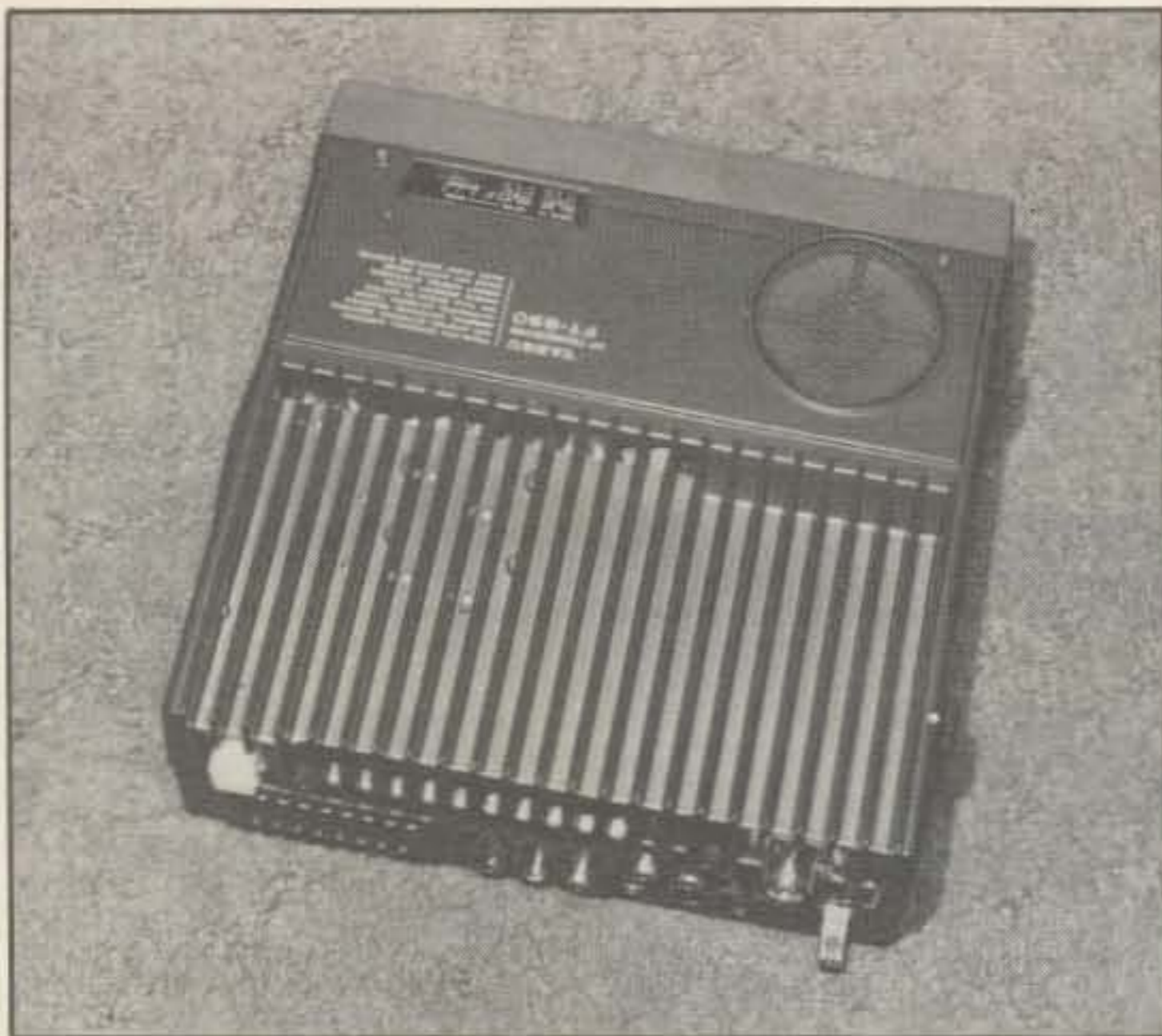
This top view shows the extremely large heatsink which is backed up by an internal fan. Air is sucked in from a vent on the rear panel and exits to the rear of the heatsink. The small internal speaker is obvious. To the left of it and towards the front panel are the top-mounted keyer controls.
