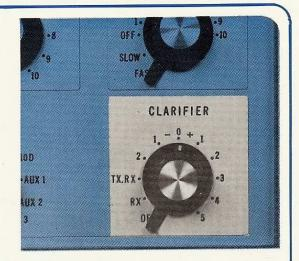
CLARIFIER CONTROL is a new feature not normally available on present amateur equipment. In the RX position this control allows the operator to vary only the receiver frepuency  $\pm$  5KC for sharp signal reception. The control can also be placed in the TXRX position providing simultaneous control of both transmit and receive frequencies over a 10 KC range.
