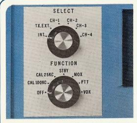
SELECT CONTROL offers choice of internal or external VFO in addition to four switched crystal controlled positions for convenient preset channel operation.
