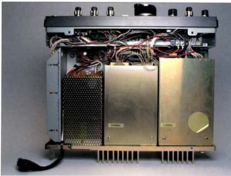
● Underside of the transceiver, with screening panels mounted.
