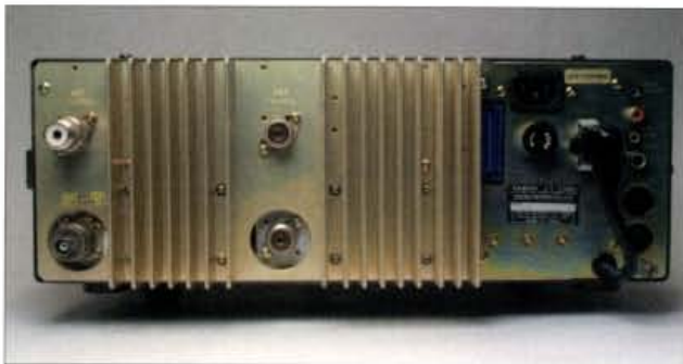
● The rear panel on the FT-736R. Although the transceiver has a relatively low power output compared to equipment manufactured today, the heat-sinking cooling fins are prominent.
