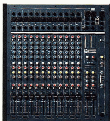
SR12 stereo and mono outputs, 12 input channels
