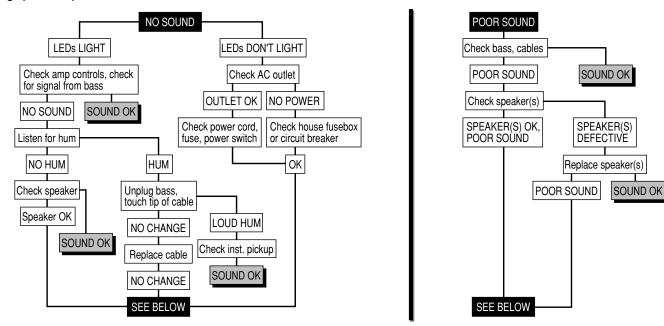
If the problem isn't covered above, or if the steps lead you here, then contact your Ampeg dealer for service information. Also, you should refer your amp to an authorized service center for servicing if it gets dropped, has liquid spilled into it, or sustains damage to its power cord.
