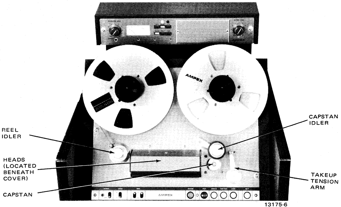
Figure 6-1. Location of Parts, Top of Transport
