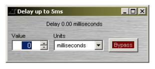
Value determines the amount of delay, based on the selected Units. Units selects either time (milliseconds) or distance (meters, centimeters, feet, or inches). Bypass disables the Delay without changing settings.
