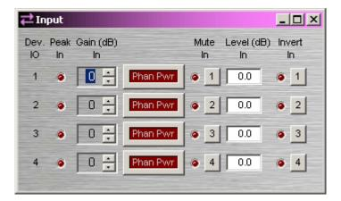
**Device IO** indicates which hardware input is associated with that software channel. **Gain In** compensates for different input signal levels, and should be set so **Peak In** flashes only occasionally (6dB headroom). **Phan Pwr** assigns +48 Volt phantom power to the input for condenser microphones. **Mute In** turns the input signal on/off. **Level In** adjusts the relative input volume. **Invert In** reverses polarity (phase) of the input signal.
