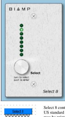
The Select 8 is an external control device, which allows initiation of eight selectable Audia actions. Actions can be individual or grouped functions within Audia. This includes recalling presets, ducking, combining, etc.
