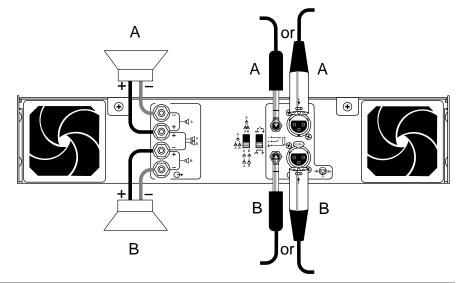
Parallel Mode Connections (5-Way Output Binding Posts)
