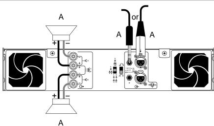
**Bridged Mono Mode Connections** (5-Way Output Binding Posts)
