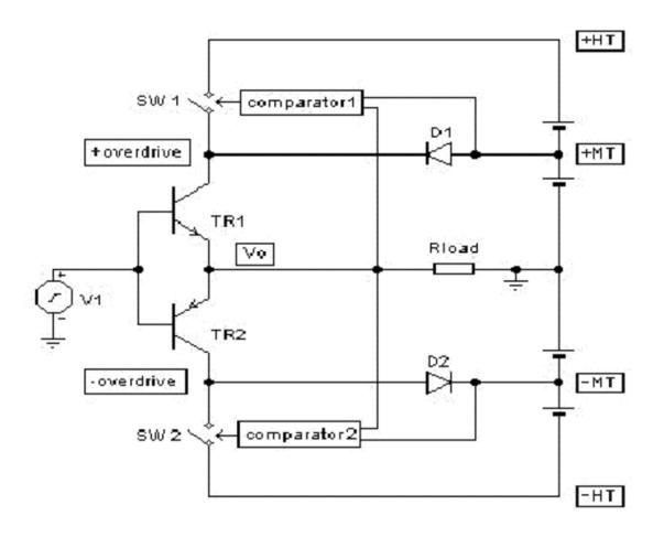
While  $V_o$  is between +MT and -MT, SW1 and SW2 are open and power is drawn from +MT and -MT through D1 and D2. If  $V_o$  gets too close to +MT, comparator1 closes SW1. Power is then drawn directly from +HT and D1 is reverse-biased. Similarly, if  $V_o$  gets too close to -MT, comparator2 closes SW2. Power is then drawn from -HT and D2 is reverse-biased.
