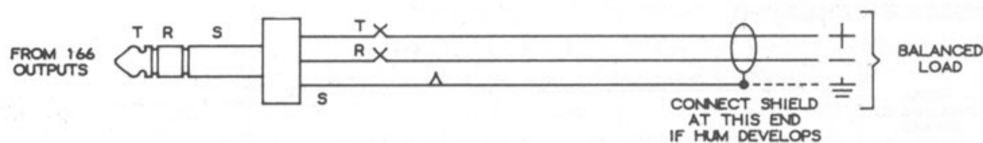
Figure 4: Balanced ins and outs, dual-conductor shielded cable, stereo plug
