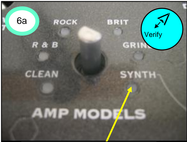
LED cover tips flush with front surface of metal (6 PL)
