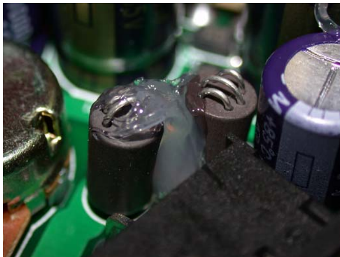
Figure #3: Add RTV between L1 and L2
