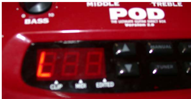
Figure # 9: “L” on the display indicates unit up-dating firmware.
