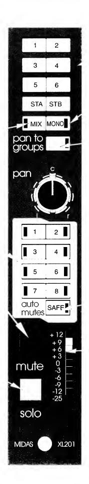
AUDIO GROUP ASSIGNS Switches 1-6 route an input channel to any of the six mono audio sub groups. Switches STA and STB route an input channel to either of the stereo audio sub groups.
