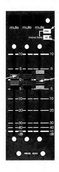
PRE Allows the signal feed from the main Left/Right outputs to the Mono output to be pre-fader rather than post-fader.
