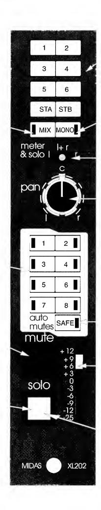
AUDIO GROUP ASSIGNS. Switches 1-6 route the input channel to the six mono audio sub groups. The left channel routing to odd groups (1,3,5) and the right channel routing to even groups (2,4,6). Switches STA and STB route the input channel in stereo to either of the stereo audio sub groups.
