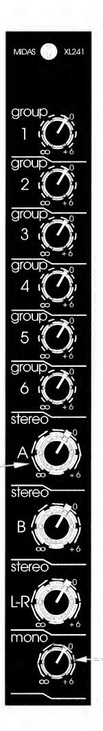
Adjusts the level of the post fader stereo Group A signal input to the matrix. Similarly for stereo B and stereo L - R (in
