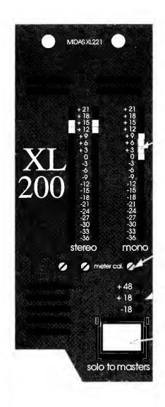
MONITOR METERS Three meters indicate left, right and mono, solo and PFL levels.
