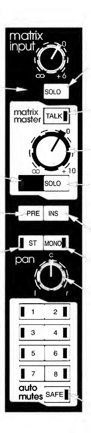
SOLO Solo's the Matrix signal to the main monitors (headphones or loudspeakers), with flashing LED indication.
