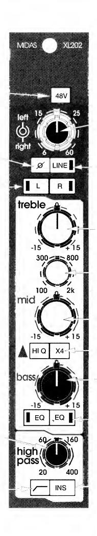
GAIN. The gain control is a wide range rotary potentiometer. The gain can be adjusted from 6dB to 60dB.
