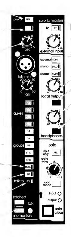
ST Connects the external input to the master left and right bus. EXTERNAL INPUT LEVEL Adjusts the level of the External Input.
