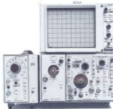
Fig. 8. TEKTRONIX 5L4N Audio Spectrum Analyzer and SG 502 Audio Oscillator
