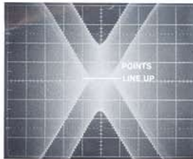
Fig. 30. Left Minus Right (L-R) Signal Used to Check Pilot Phase
