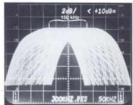
Fig. 28. Self-Sweeping an Fm Transmitter
