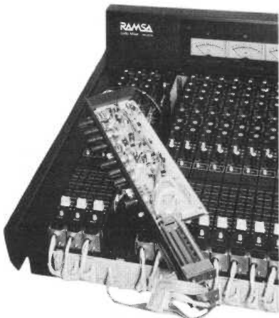
Photograph 3. Connection of the Test Cord
