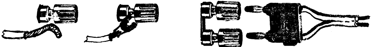
FIGURE 2-4. USE OF FIVE-WAY BINDING POSTS.
