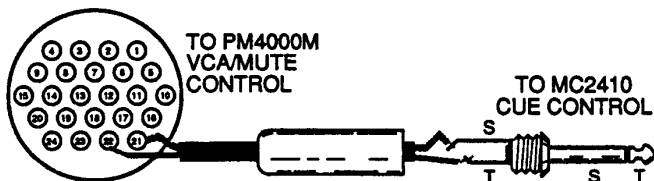
Figure 8-11. Custom Cable to Join the Cue Control Functions of the MC2410 and PM4000M
