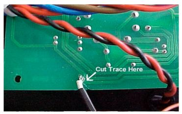
Solder the other end of the shielded cable (see picture for length) to C140/R157/V3,pin 2.
