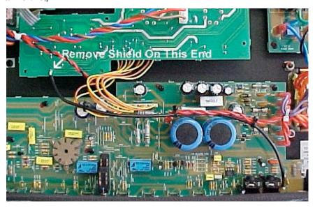
Remove the shield from the cable on the power amp side.
