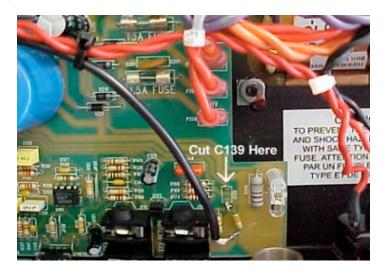
Cut signal trace to C140/R157/V3,pin 2 on power amp just before reaches any components.
