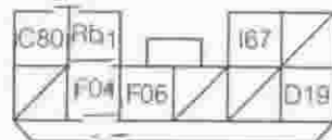
61g : Floor wire No. 1 (To junction block I)
