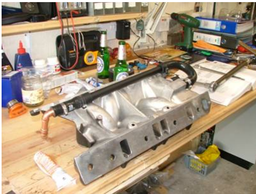
Figure 16 – Underside of injection manifold
