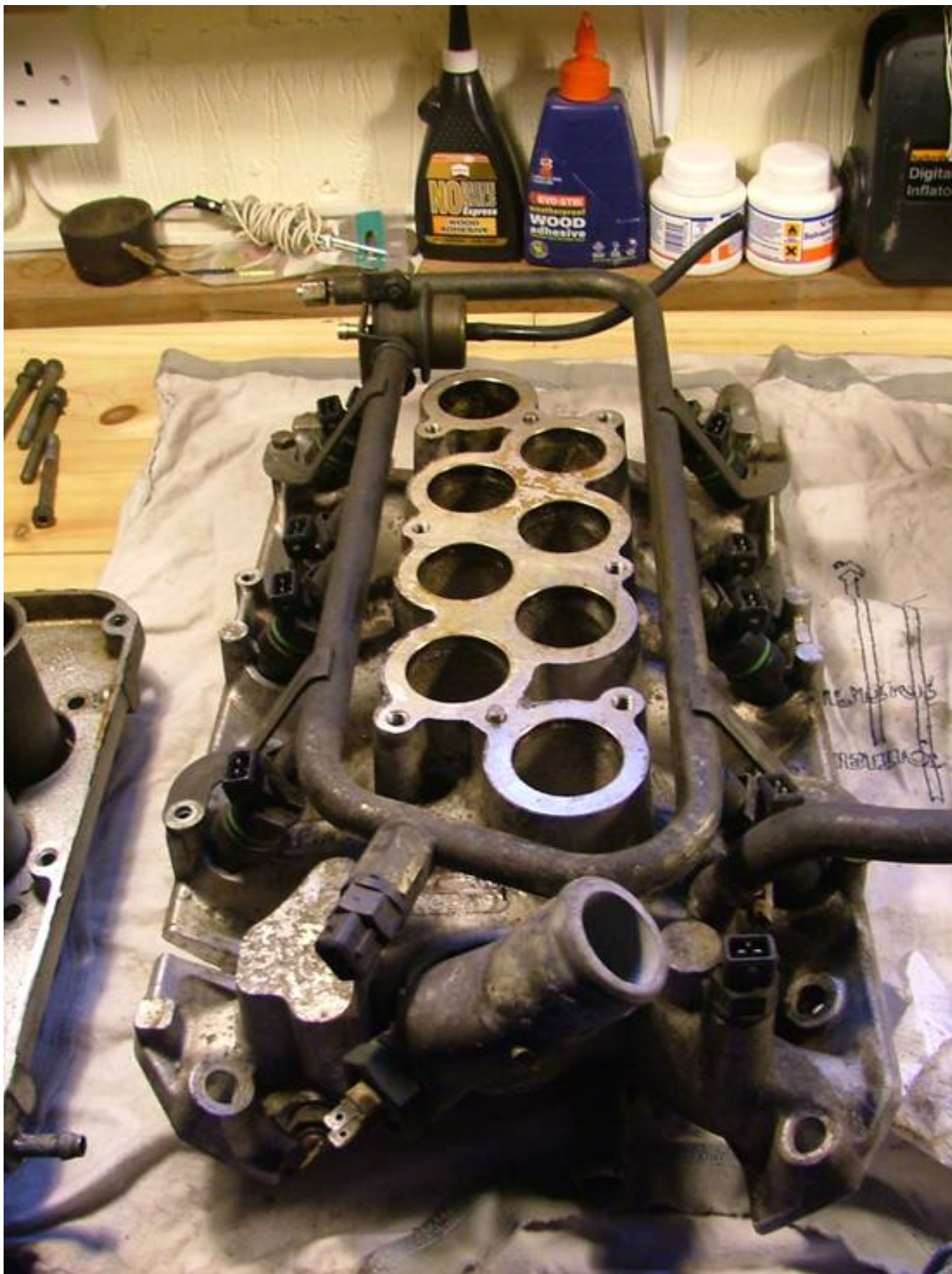
Figure 4 – View of stripped intake manifold
