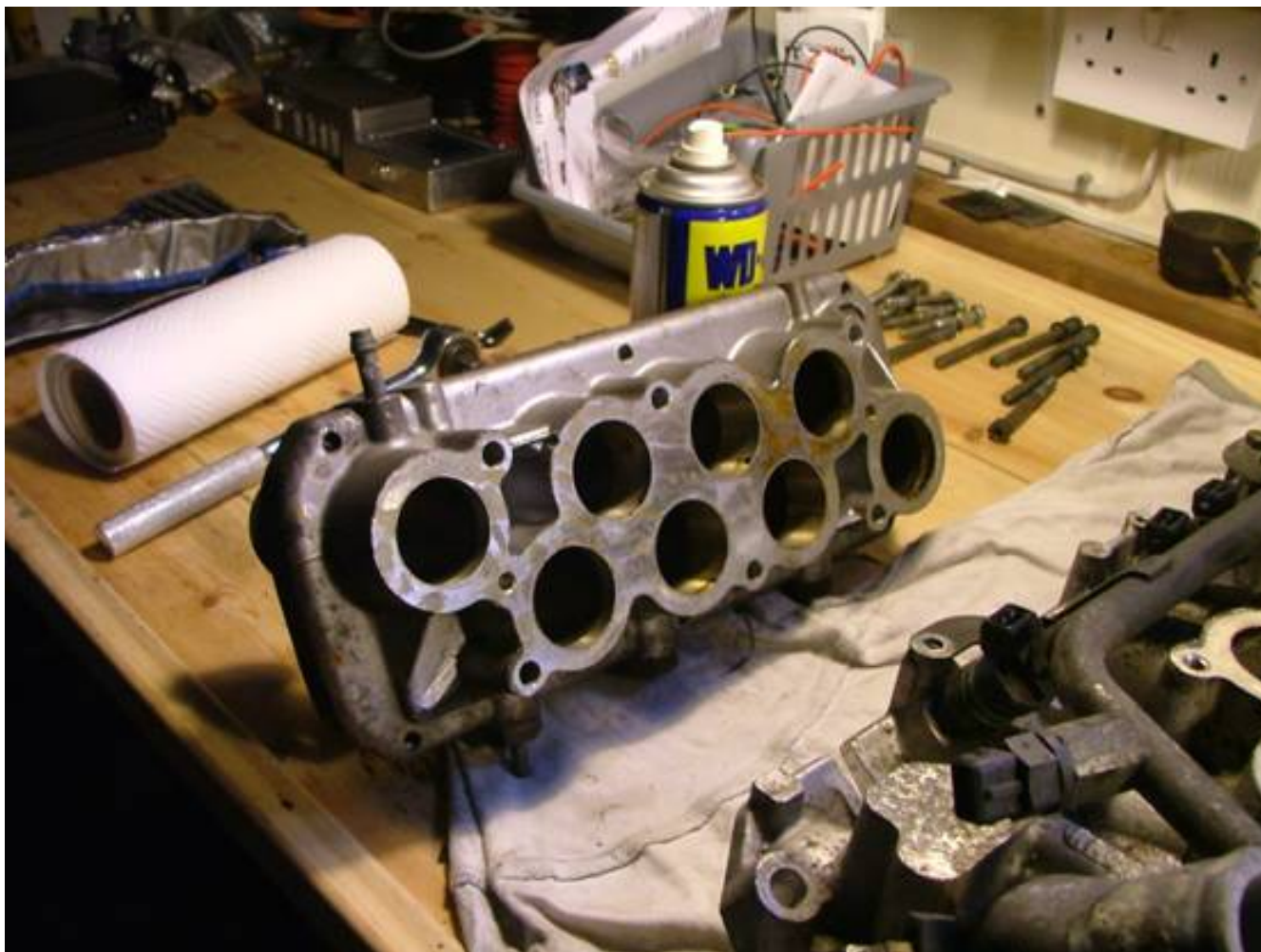
Figure 21 – Underside of plenum intake trumpet housing (note vacuum ports)
