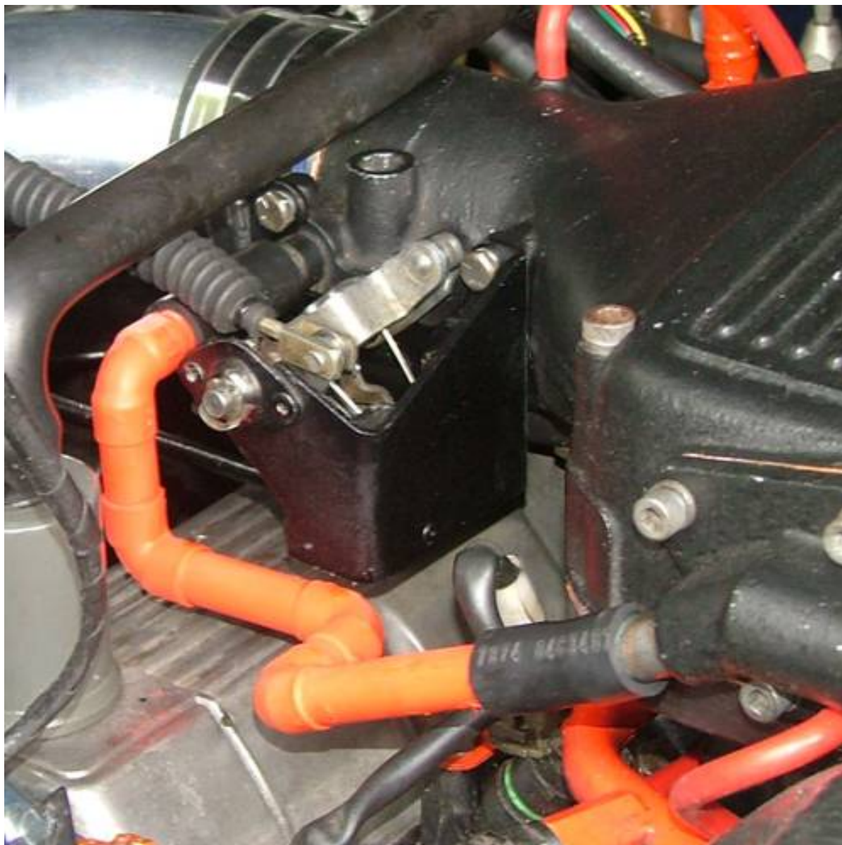
Figure 37 – Idle air supply pipe (red) – finalised
