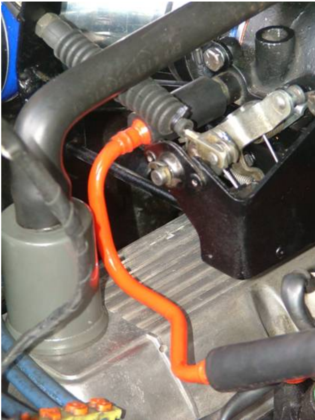
Figure 36 – Idle air supply pipe (red) – no longer used
