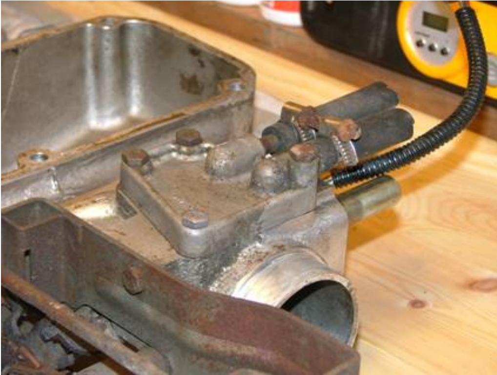
Figure 7 – Close up of plenum chamber pre-heater
