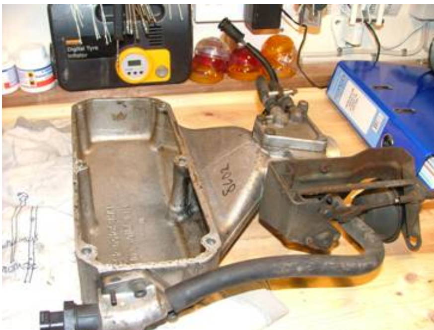
Figure 6 – Underside of plenum.
