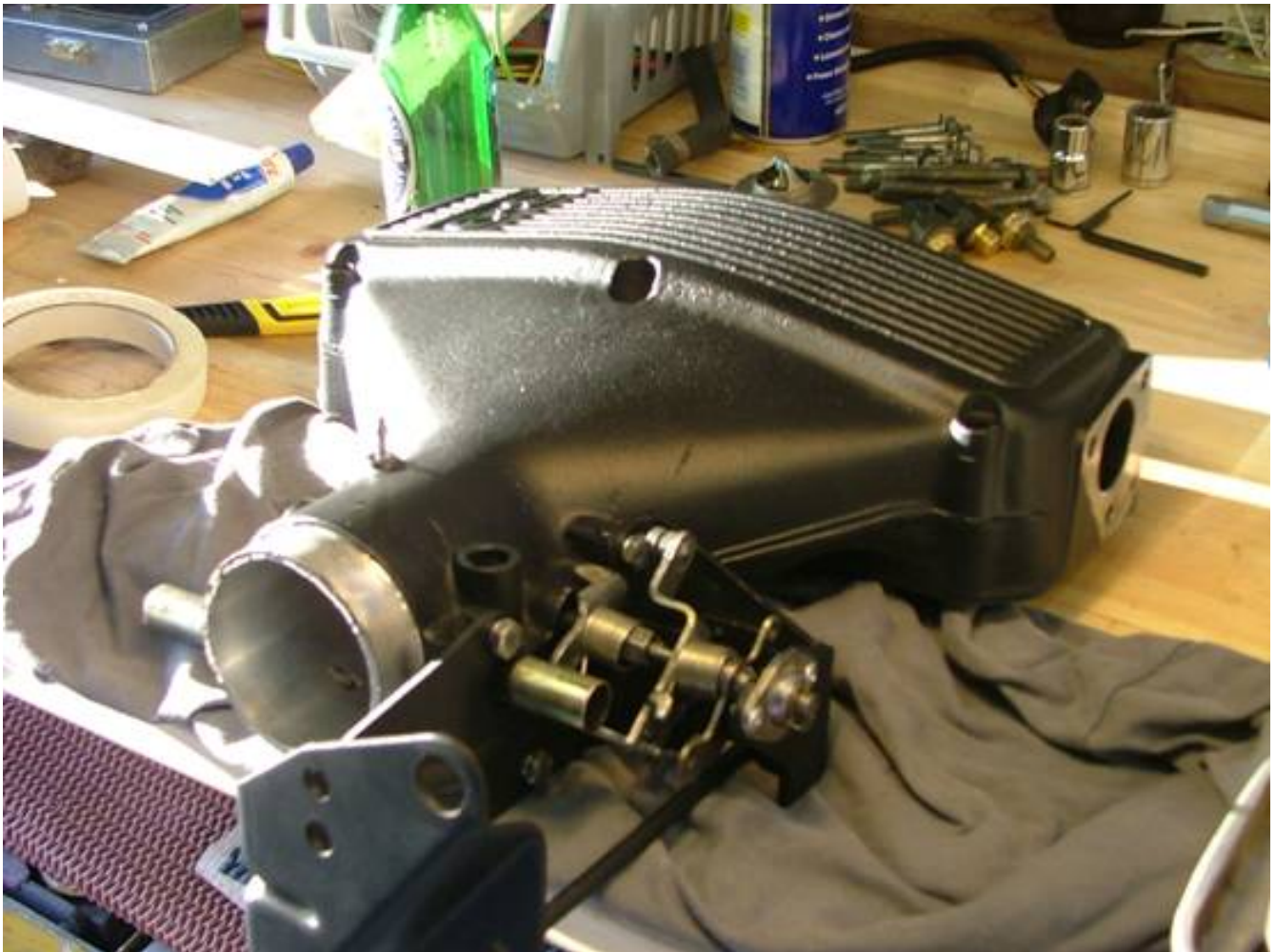
Figure 12 – Sprayed plenum complete with rebuilt throttle linkages
