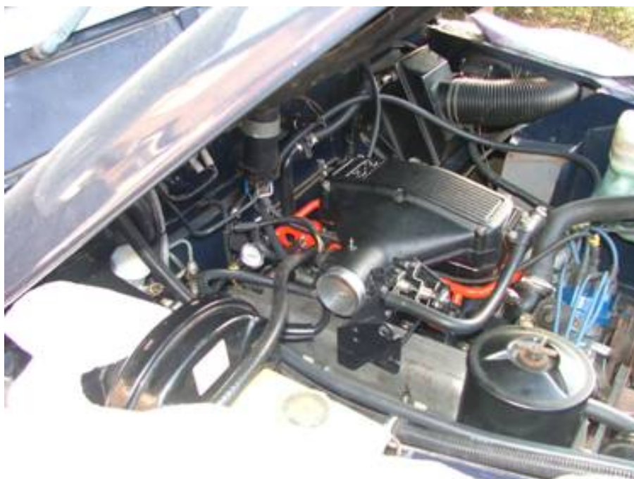
Figure 22 – Final position of the plenum
