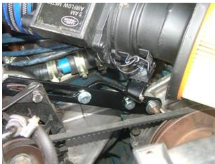
Figure 27 – MAFS mounting bracket
