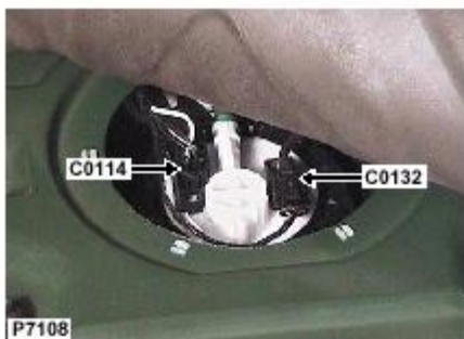
Description: Unit-Fuel Tank Location: Beneath fuel tank cover
