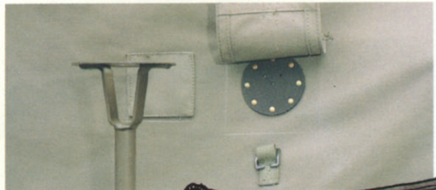
Aerial outlet and support brackets.
