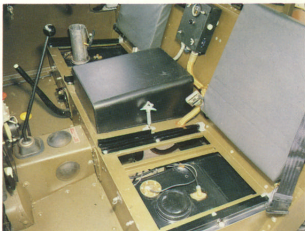
Twin underseat fuel tanks.
