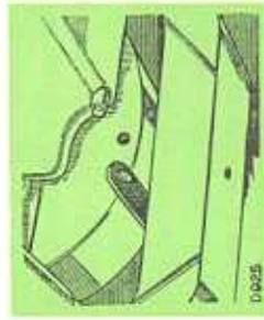
Flywheel housing drain plug
