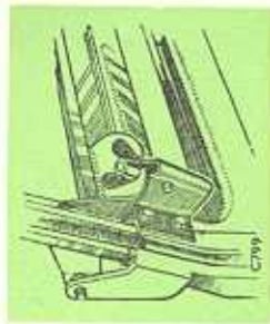
Windscreen fixing screws
