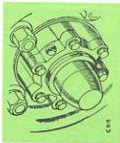
Oil filler plug, rear axle hub
