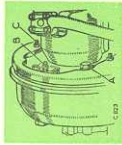
Wheel brake adjustment
