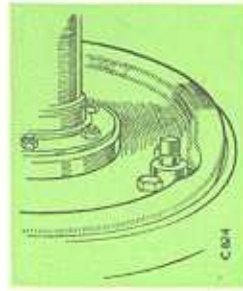
Wheel brake adjustment
