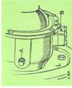
Swivel pin housing lubrication A—Filler/level plug B—Drain plug
