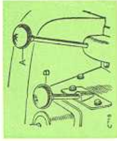
Transfer gear change lever, and front wheel drive control A—Transfer gear change lever B—Front wheel drive control
