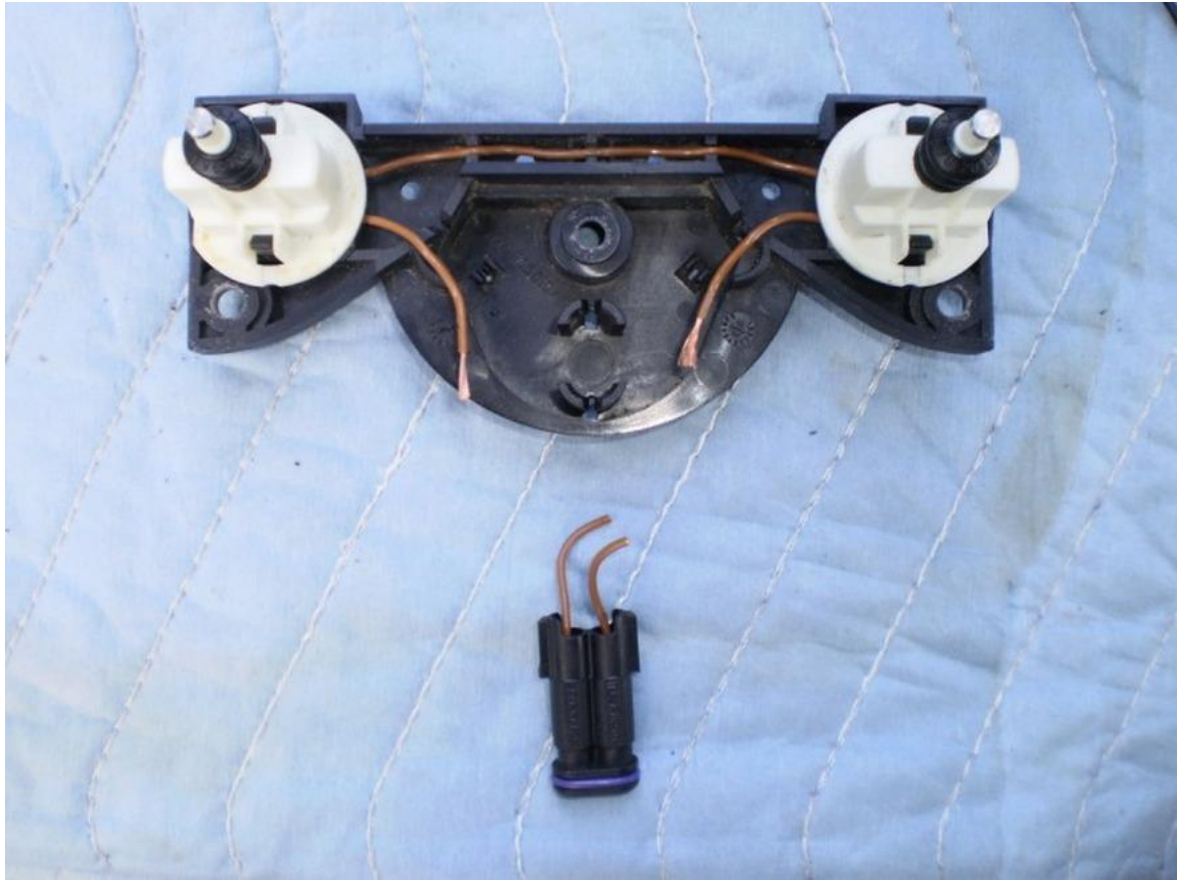
39. Splice, solder, and heat shrink the longer end of the trailer connector to the SVS wires and run them through the SVS cover plate.
