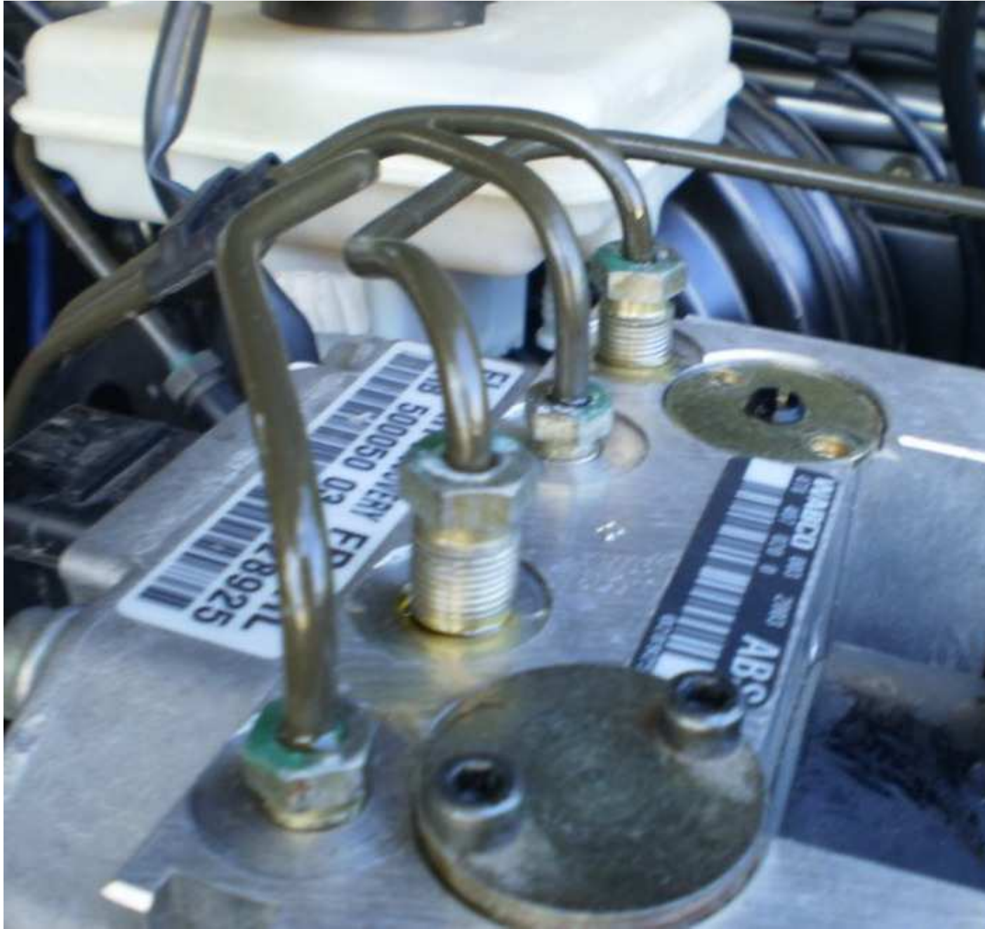
10. Unscrew and disconnect the two smaller brake lines. Brake fluid will be dispensed from both the lines and pump side. Have a second shop towel nearby.
