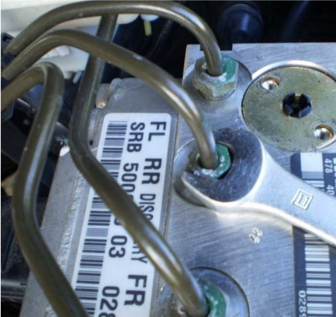
7. Brake loose the two side mounted brake line nuts using a 13mm wrench.
