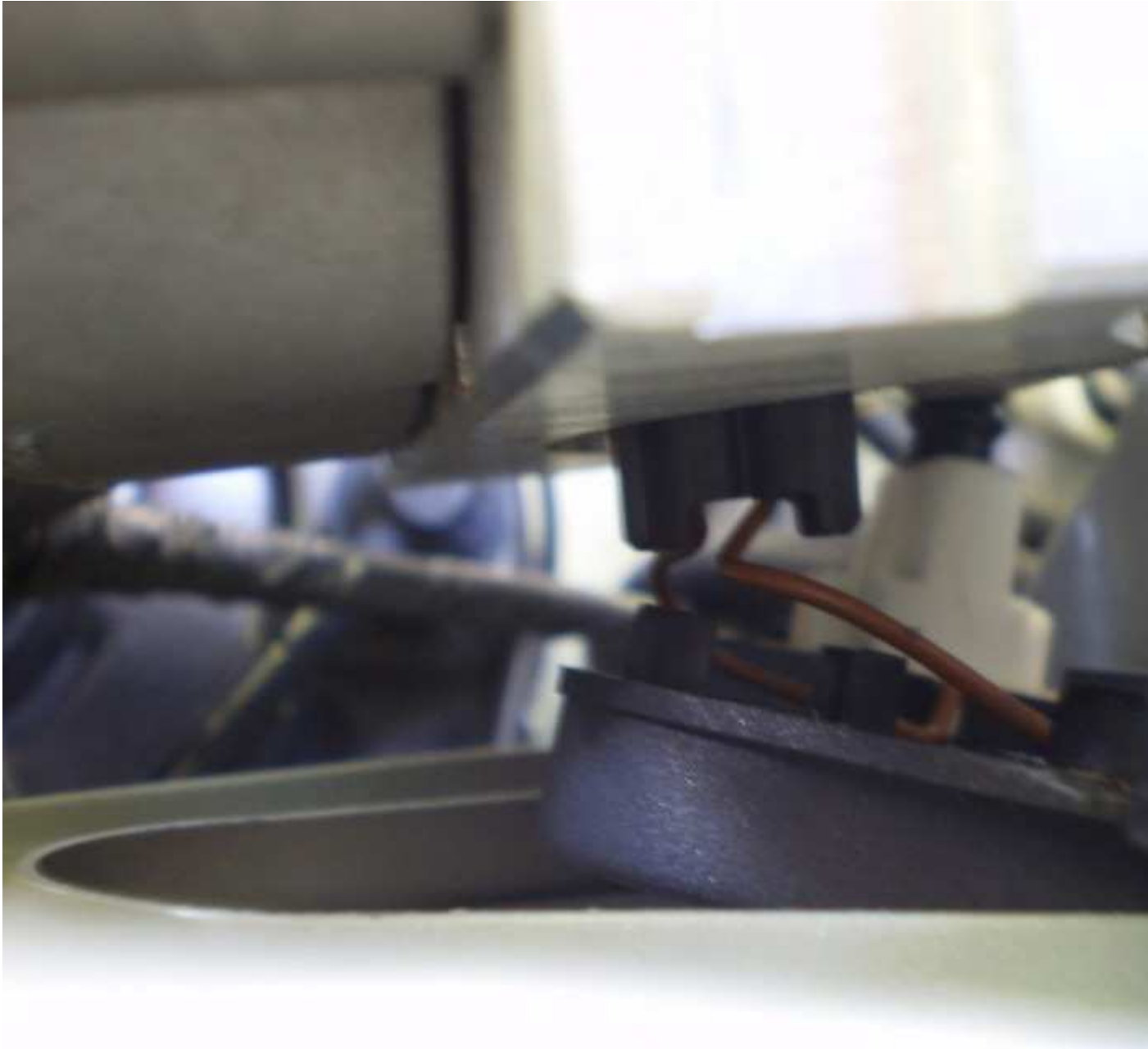
29. You should have enough room to get your fingers underneath and pull the SVS plug down. I needed my assistant to raise the ABS modulator/pump an inch or two so I could use my thumb to unplug it.
