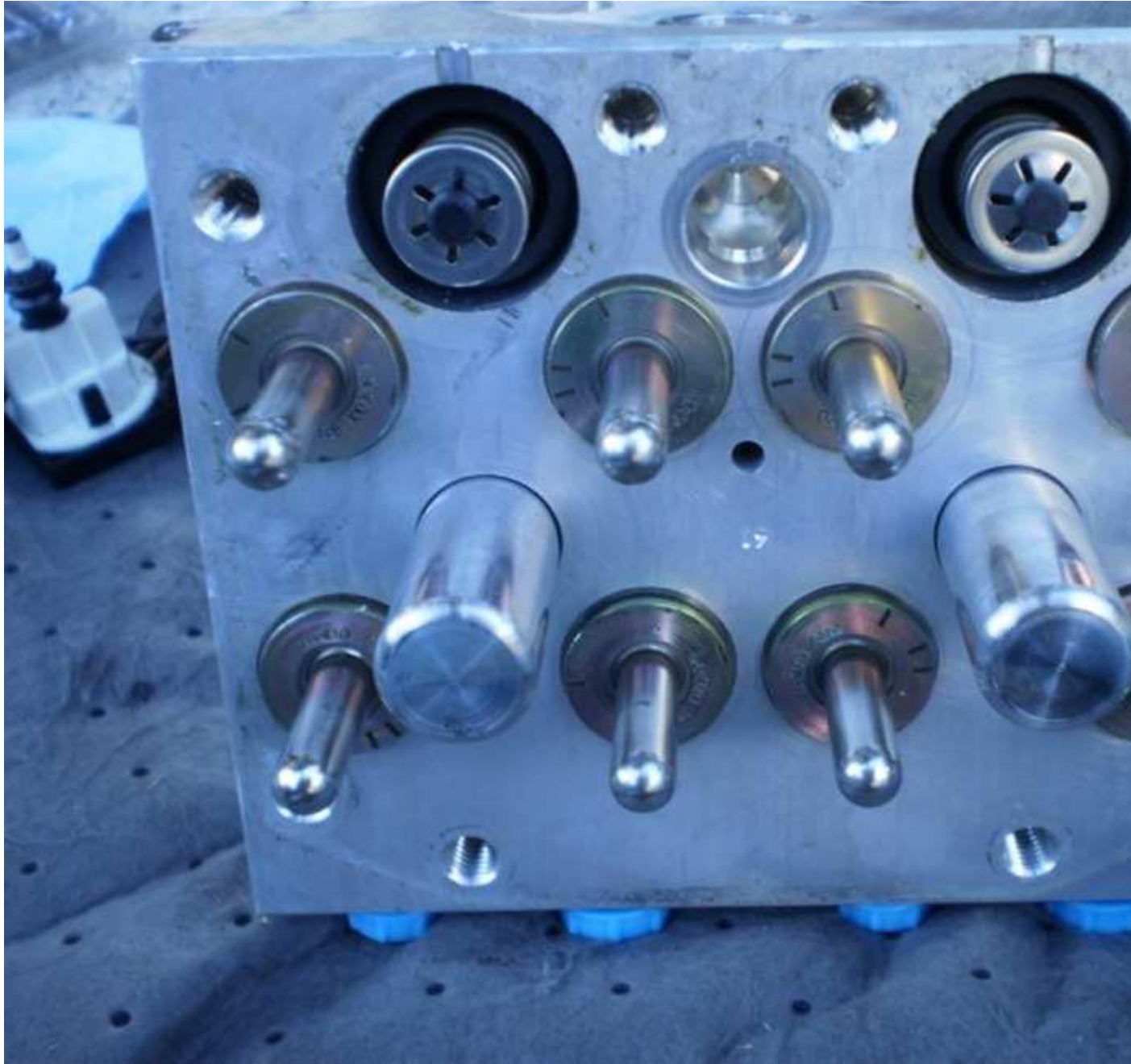
Pump side of the unit. Unit is upside down. Notice the brake line plugs at bottom.
