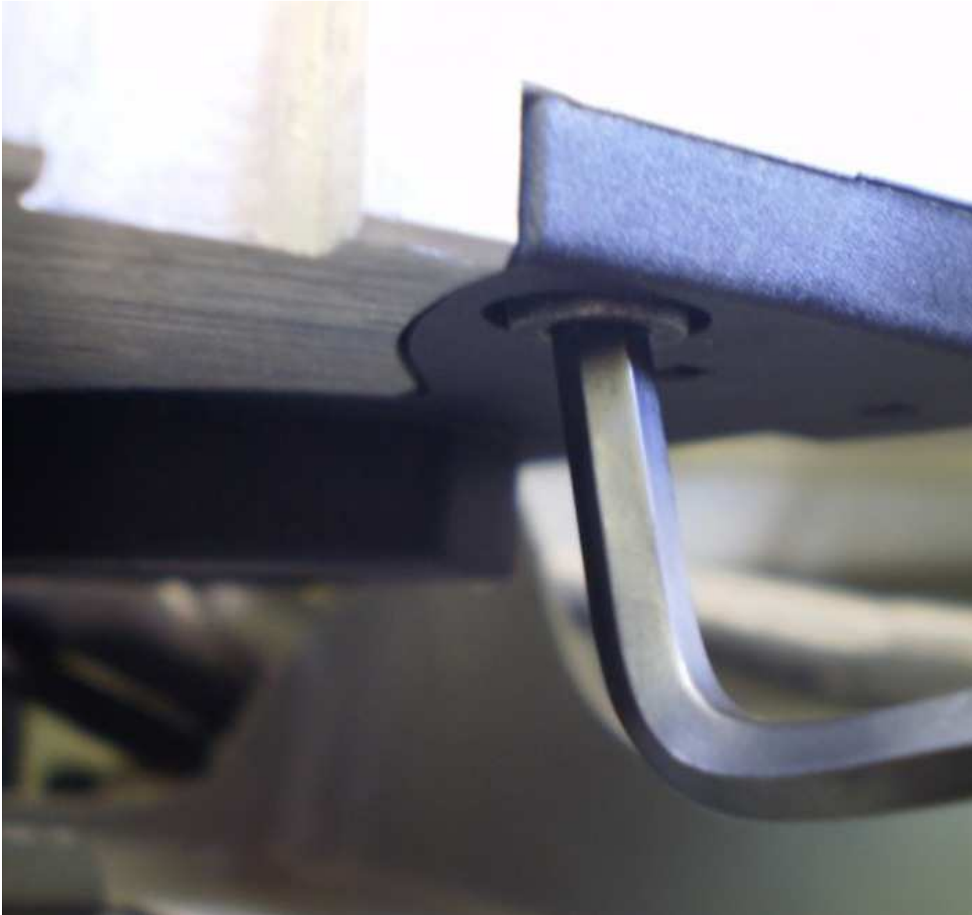
28. Once all three screws are out, carefully pry down the SVS cover plate.
