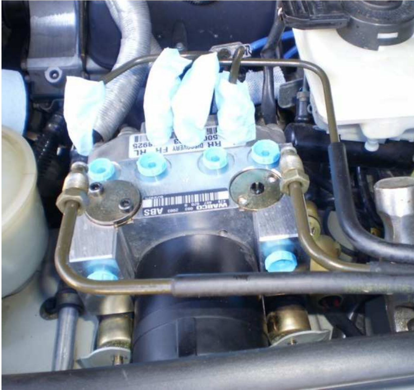
12. Lift the front of the modulator and remove the front rubber mount.
