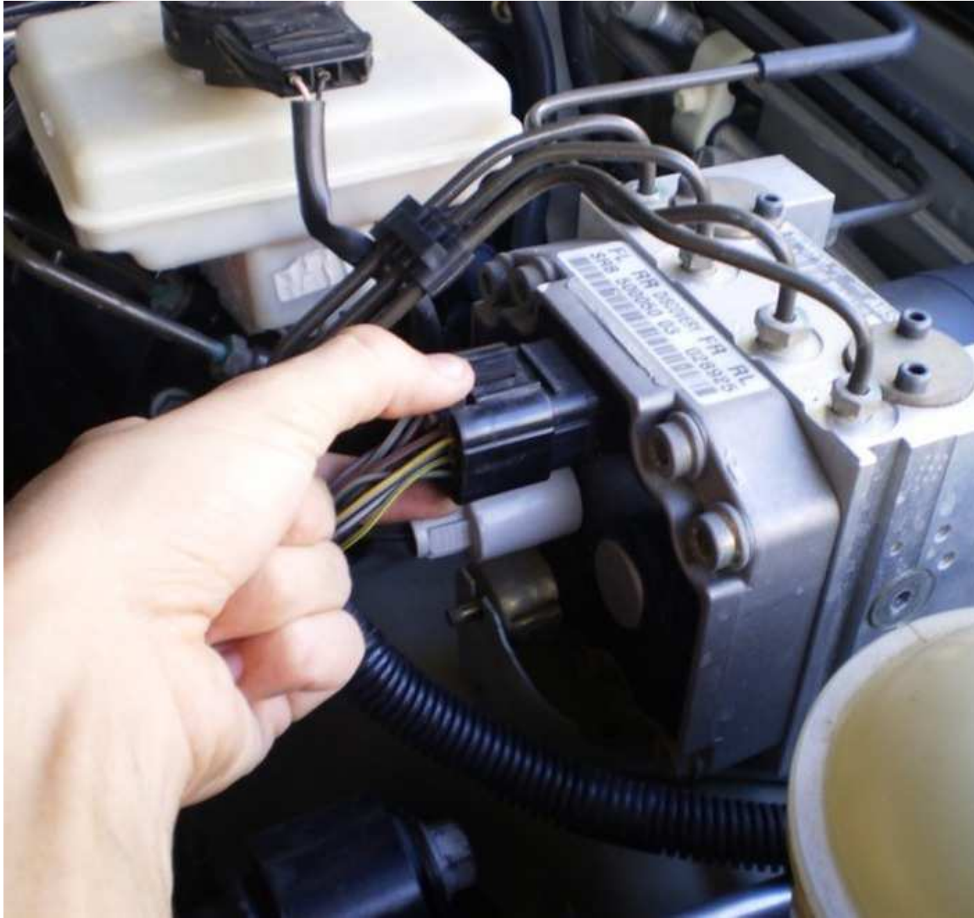
Removing black connector C0501 and grey connector C0500
