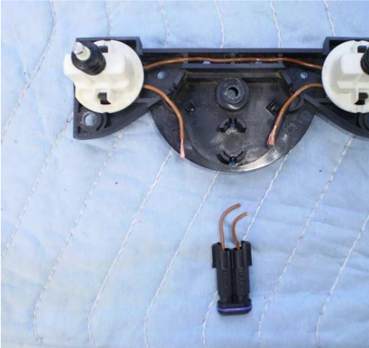
39. Splice, solder, and heat shrink the longer end of the trailer connector to the SVS wires and run them through the SVS cover plate.
